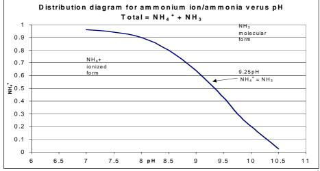
The HI 7609829-10 sensor is specified for 0.02 to 200 ppm (mg/L)  $NH_4^+$ -N (equivalent to 0.026-260 ppm (mg/L)  $NH_4^+$ ). Based on the corresponding molecular weights of nitrogen and ammonium, the relationship is:  $NH_4^-$ -N = ( $NH_4^+$ )(14/18) = ( $NH_4^+$ ) x 0.7778.  $NH_4^+$ -N is also called ionized ammonia. The sensor responds in a Nernstian manner (like a pH sensor) and produces a voltage that the meter converts to a concentration value.
