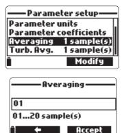
**Note** Each reading takes 1 second, so when logging the first sample will be delayed by a few seconds if averaging is used.
